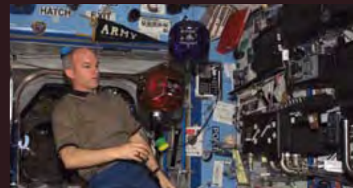
SPHERES are innovative micro-satellites designed for operations in microgravity by the MIT Space Systems Laboratory in cooperation with Payload Systems Inc. Here, astronaut Jeff Williams is performing autonomous formation flight testing aboard the International Space Station during Expedition 13 in 2006.
